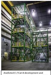
Anellotech's TCat-8 development and testing unit for converting biomass to BTX. Photo courtesy of Zeton Inc.
